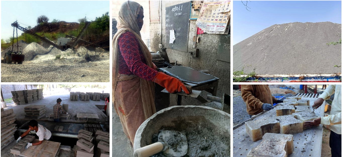
The process of reusing stone crusher dust as manufacturing sand
