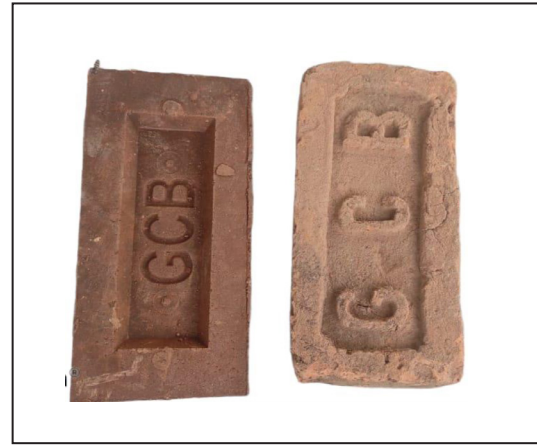
Difference of quality between good bricks and locally made bricks
