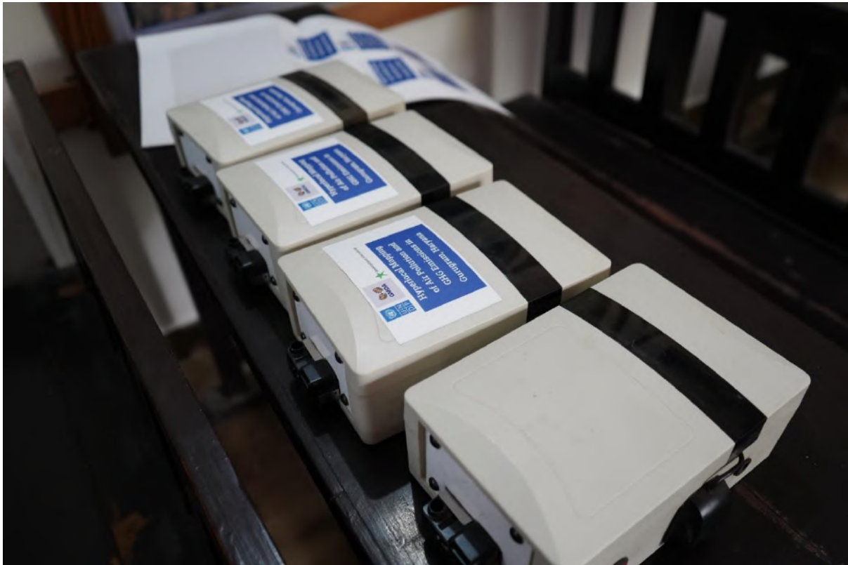
Air Quality Monitoring Sensor (IoT)
