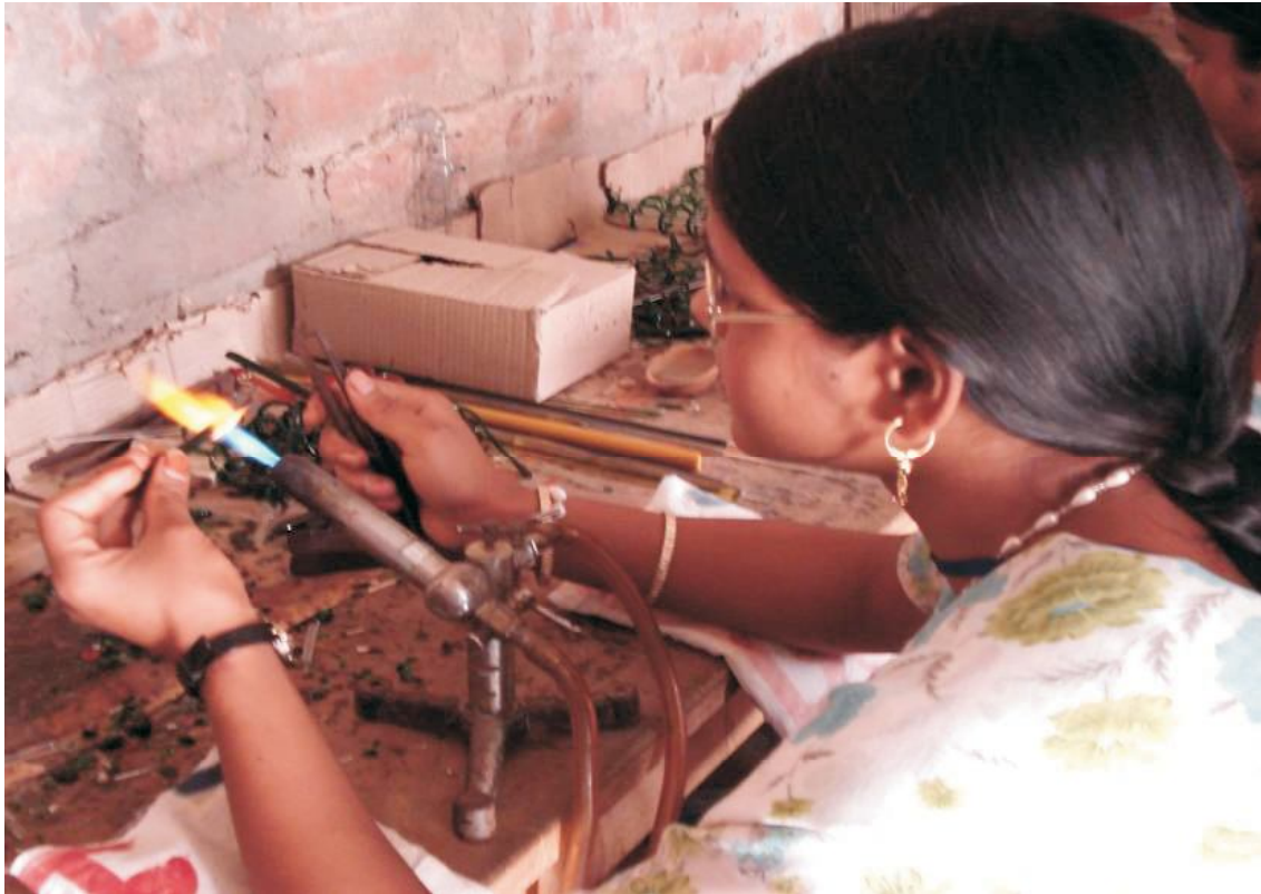
The jodai (joining process ) being performed by a woman worker.
