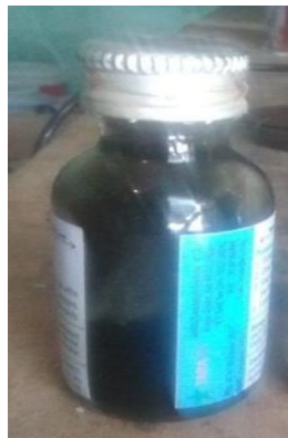
Vial testing – tested raw water turned black indicating bacterial contamination in raw water sample.
