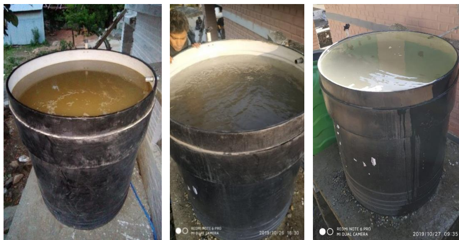
Quality of water in filter tank at three stages- left: after 2 hrs of backwashing, middle: after 6-7hrs of backwashing, right: after 12 hrs of backwashing.
