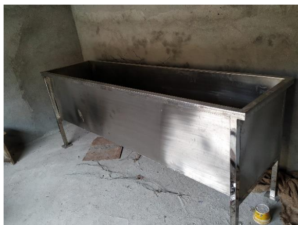
Stainless steel tank for dipping the wood in preservative. Size 8'x2'x2'
