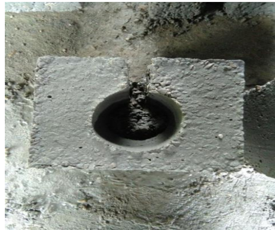
Type 5 -Hollow concrete half block of size – 6 inch x 8 inch x 6 inch with cavity at 8 inch edge.
