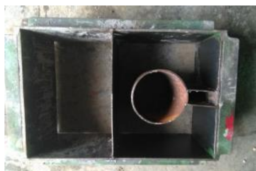
Moulds for solid concrete block block with cavity for vertical reinforcement
