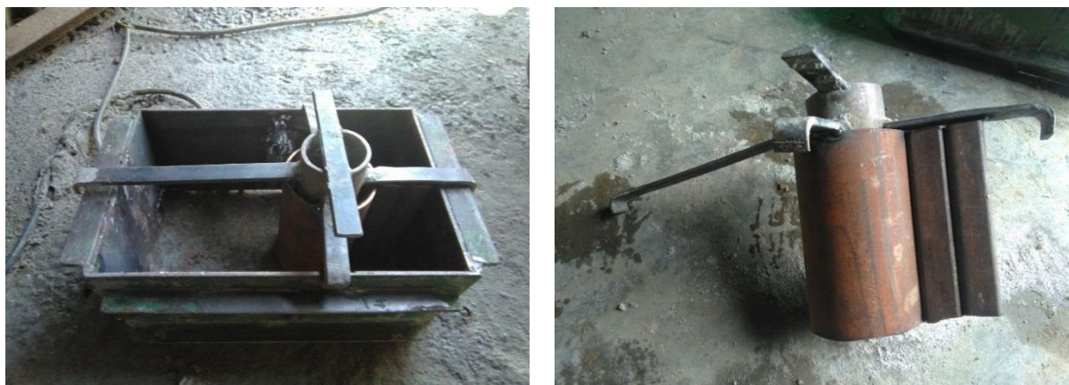
Accessories for demoulding of cavity block
