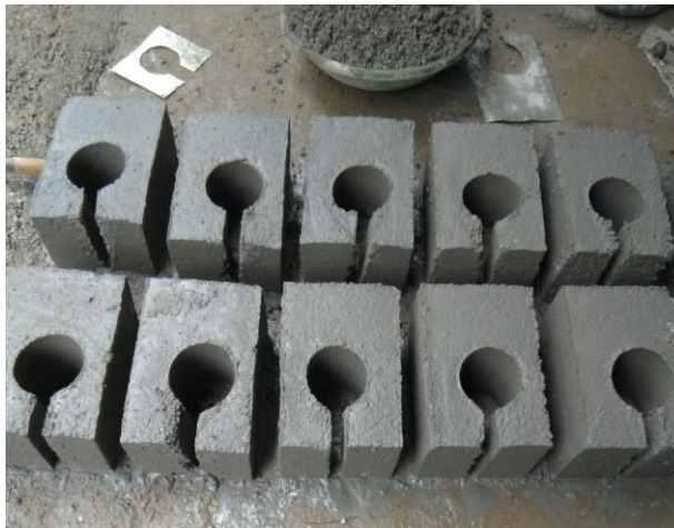
Type 4 -Hollow concrete block of size – 12 inch x 8 inch x 6 inch for corner junctions.
