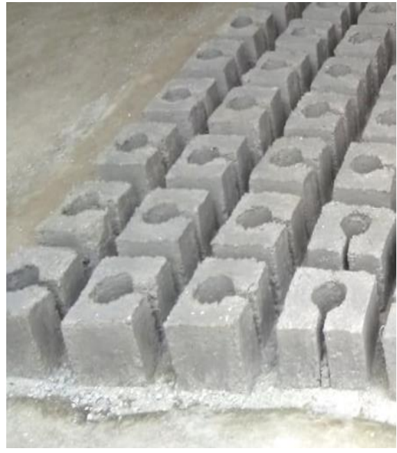
Type 3 and Type 6 of hollow concrete half blocks-at left side 12 inch x 8 inch x 6 inch with cavity at 12 inch side for T-junctions and right side 6 inch x 8 inch x 6 inch half block with cavity at 6 inch edge.
