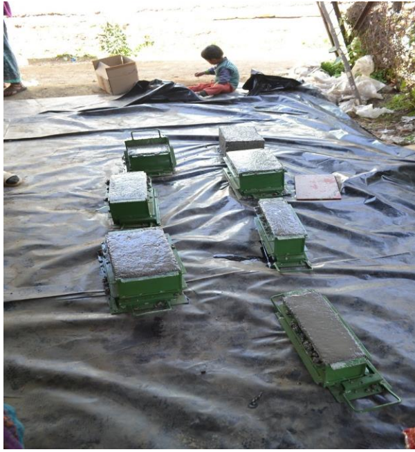
Type 1 and Type 2 Solid concrete blocks – 12 inch x 8 inch x 6 inch for external wall and 12 inch x 4 inch x 6 inch for internal partition wall.
