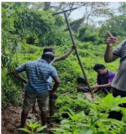
Clay sampling with a 5m manual drill
