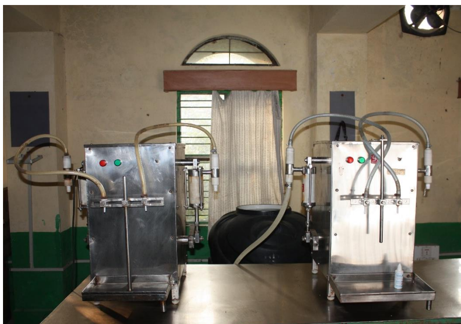
Figure 4 Production Centre at Orchha with 2 Maxi WATA devices
